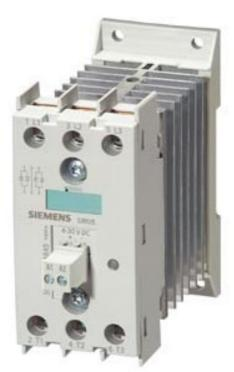
Solid-state contactor 3-phase 3RF2 AC 51 / 10 A / 40  $^{\circ}\text{C}$  48-600 V / 4-30 V DC 2-phase controlled screw terminal Blocking voltage 1200 V
