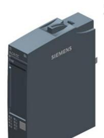
SIMATIC ET 200SP, Digital input module, DI 8x 24V DC SRC BA, type 1 (IEC 61131), source Input (NPN, M-reading) Packing unit: 1 piece, fits to BU-type A0, Colour Code CC02, input delay time 0,05..20ms, module diagnostics for: supply voltage
