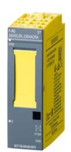
SIMATIC DP, ELECTRON. MODULE FOR ET200SP, F-RQ 1X24VDC/24..230VAC/5A ST, 20MM WIDTH, 1 RELAY OUTPUT (2 NO-CONTACTS) TOTAL OUTPUT CURRENT 5A, RATED VOLTAGE DC 24V AND AC 24 .. 230V, USEABLE UP TO PL E (ISO13849-1: 2008)/ SIL 3 (IEC61508: 2010) IF CONTROLLED BY A F-DQ (E.G. 6ES7136-6DB00-0CA0)
