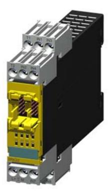
SIRIUS, Extension module 3RK32 for modular Safety system 3RK3 4/8 F-DI, 24 V DC Can be parameterized via MSS ES 22.5 mm overall width screw terminal Up to SIL3 (IEC 61508) Up to Performance Level E (ISO 13849-1) without connection cable
