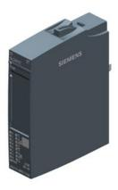
SIPLUS ET 200SP DI 8x24 V DC SRC BA based on 6ES7131-6BF61-0AA0 with conformal coating, -40...+70 °C, digital input module, suitable for BU type A0, color code CC02, source input, (NPN, sourcing input) input type 1 (IEC 61131), input delay 0.05..20 ms module diagnostics for: supply voltage
