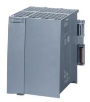
SIMATIC S7-1500, System power supply with buffer functionality PS 60W 24/48/60V DC HF, supplies the backplane bus of the S7-1500 with operating voltage and permits the CPU to retain RAM (data) retentively
