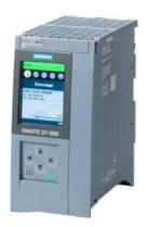
SIMATIC S7-1500, CPU 1516-3 PN/DP, central processing unit with 2 MB work memory for program and 7.5 MB for data 1st interface: PROFINET IRT with 2-port switch, 2nd interface: PROFINET RT, 3rd interface: PROFIBUS, 6 ns bit performance, SIMATIC Memory Card required \*\*\* approvals and certificates according to entry 109816732 at support.industry.siemens.com to be considered! \*\*\*
