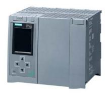
SIMATIC S7-1500F, CPU 1517F-3 PN/DP, Central processing unit with Work memory 3 MB for Program and 8 MB for data, 1st interface: PROFINET IRT with 2-port switch, 2nd interface: PROFINET RT, 3rd interface: PROFIBUS, 2 ns bit performance, SIMATIC Memory Card required
