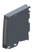
SIMATIC S7-1500 Analog input/output module AI 4x U/I/R/RTD/TC ST; 4 channels in groups of 4; Hardware interrupts; Diagnostics AQ 2x U/I ST; 2 channels in groups of 2; Substitute value; Diagnostics Common mode voltage approx. 10 V 16 bit; Accuracy 0.3%; Delivery including push-in front connector, infeed element, shield bracket and shield terminal
