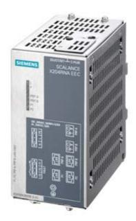
SCALANCE X204RNA EEC; redundant network access 2x 100 Mbit/s RJ45 ports; 2x 100 Mbit/s combo ports; LED diagnostics; error signaling contact with set button; simple power supply; network management; incl. electronic manual on CD-ROM, C-plug optional for HSR network;
