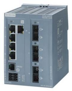
Preset for Ethernet/IP mode! SCALANCE XB205-3LD managed Layer 2 IE Switch 5x 10/100 Mbit/s RJ45 ports 3x SM FO SC port 1x console port, diagnostics LED redundant power supply; Temp. range 0 °C to +60 °C; Mounting onto standard rail; Default EtherNet/IP
