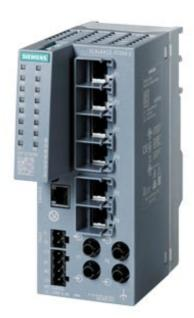
SCALANCE XC206-2 manageable layer 2 IE Switch; 6x 100 Mbit/s RJ45 ports; 2x 100 Mbit/s ST/BFOC ports; 1x console port; Diagnostic LED; Redundant power supply; Temp. range -40°C to +70 °C Mounting: Standard Mounting Rail/S7 Profile Rail/Wall redundancy functions; office features (RSTP, VLAN ,...); PROFINET IO Device; Ethernet/IP-compliant C-PLUG-shaft;
