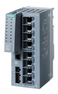
SCALANCE XC208 manageable layer 2 IE Switch; 8x 10/100 Mbit/s RJ45 ports; 1x console port; Diagnostic LED; Redundant power supply; Temp. range -40°C to +70 °C Mounting: Standard Mounting Rail/S7 Profile Rail/Wall Office redundancy functions features (RSTP, VLAN ,...); PROFINET IO device Ethernet/IP-compliant C-PLUG shaft;
