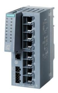
SCALANCE XC208G Manageable layer 2 IE switch; 8x 10/100/1000 Mbit/s; RJ45 ports; 1x console port; Diagnostics LED; Redundant power supply; Temp. range -40 °C to +70 °C Mounting: Standard mounting rail/S7 mounting rail/wall; Redundancy functions; Office features (RSTP, VLAN,...); PROFINET IO device; Ethernet/IP-compliant; C-PLUG slot;
