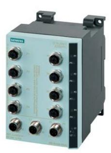
SCALANCE X208PRO, managed IE switch, 8x 10/100 Mbit/s M12 ports, IP65/67, LED diagnostics, error signaling contact, Redundant power supply, PROFINET IO device, network management, can be operated in redundant ring, dust caps, incl. electronic manual on CD-ROM, C-plug optional
