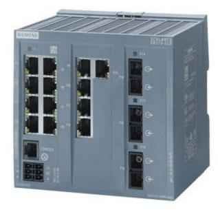
Preset for Ethernet/IP mode! SCALANCE XB213-3LD managed Layer 2 IE Switch 13x 10/100 Mbit/s RJ45 ports, 3x SM FO SC port 1x console port, diagnostics LED, redundant power supply, temp. range 0 °C to +60 °C; mounting onto standard rail; Default EtherNet/IP
