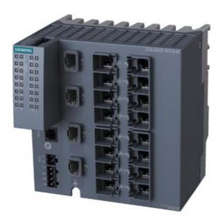
SCALANCE XC216-4C Manageable Layer 2 IE Switch; 12x 10/100 Mbit/s RJ45 ports; 4x 1000 Mbit/s combo ports (either 1000 Mbit/s SFPs or 10/100/1000 Mbit/s RJ45 ports can be used); 1x console port; diagnostics LED; Redundant power supply; Temp. range -40 °C to +70 °C Mounting: Standard mounting rail/S7 mounting rail/wall; Redundancy functions; Office features (RSTP, VLAN, etc.); PROFINET IO device; Ethernet/IP-compliant; C-PLUG slot;
