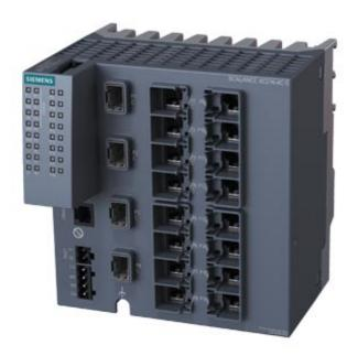
SCALANCE XC216-4C G manageable layer 2 IE Switch; Full Gigabit; 12x 10/100/1000 Mbps RJ45 ports; 4x 1000 Mbps combo ports (either 1000 Mbps s SFPs or 10/100/1000 Mbps RJ45 ports can be used); 1x console port; Diagnostic LED; redundant power supply; Temp. range -40 °C to +70 °C; Mounting: Standard mounting rail/S7 mounting rail/wall; redundancy functions; office features (RSTP, VLAN ,...); PROFINET IO Device; Ethernet/IP conformity; C-PLUG shaft;
