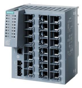
SCALANCE XC224 manageable layer 2 IE Switch; 24x 10/100 Mbit/s RJ45-Ports; 1x console port, Diagnostic LED; Redundant power supply; Temp. range -40°C to +70 °C Mounting: Standard Mounting Rail/S7 Profile Rail/Wall Office redundancy functions features (RSTP, VLAN ,...); PROFINET IO device Ethernet/IP-compliant, C-PLUG shaft;
