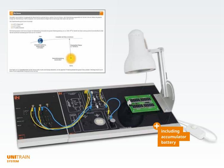
Photovoltaics is a term describing the direct conversion of sunlight into electrical energy by means of solar cells. In vehicles, energy obtained in this way is used for auxiliary electrical loads, i.e. for the comfort of drivers and passengers, for instance cooling the interior on hot sunny days. This UniTrain system helps trainees understand the technological principles behind this in rapid time.
