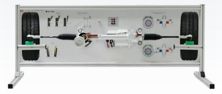
Electromechanical servo-steering offers many advantages over steering systems without such assistance. It provides not only physical, but also psychological benefits to drivers. Steering assistance is provided based on need. This means that it only becomes active when a driver wants it. Simultaneously, though, it also responds to speed, steering torque and angle.
