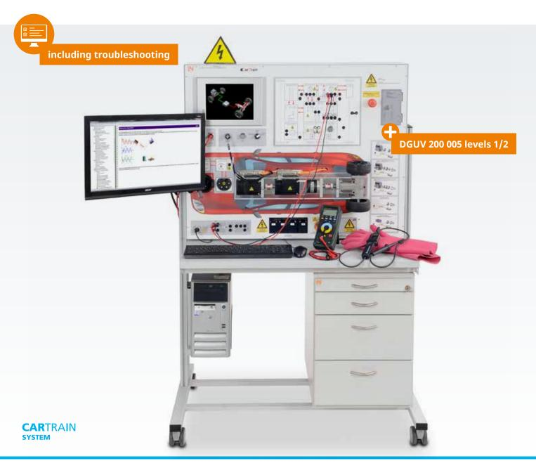
This is a world first, a CarTrain system which combines five different drive configurations, including measuring points for all electrical components of a high-voltage system in a single set.
