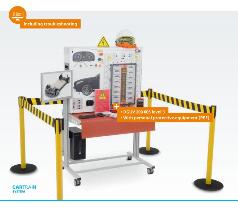
More and more manufacturers are carrying out repairs on high-voltage batteries. This is a new challenge for mechanics and requires a special understanding of the systems involved. This training system makes it possible to work directly with a real high-voltage battery. Trainees can carry out measurements inside the battery, work at cell level and even change actual cells.
