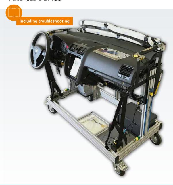
This training model provides all the necessary diagnostic skills with the help of a complete SRS system. It consists entirely of OEM components from a Volkswagen Golf 5, thus providing authentic learning experience. It also includes an on-board network control unit, original fuses and cable harness plus a full set of crash sensors. A full set of actuators is also provided, but these devices do not actually trigger so that it is possible to work with them safely.
