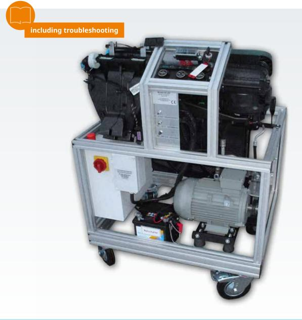
This training model conveys all the necessary diagnostic skills for two-zone air conditioning using a real two-zone system. It consists entirely of OEM components from a Volkswagen Golf 5 which allows students to go through an authentic learning experience. Even connection of an air conditioning service station to a complete refrigerant circuit with expansion valve is not a problem.
