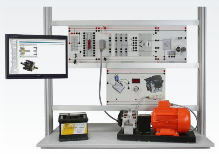
Our system enables trainees to become familiar with the function of a hybrid controller. They can experiment for themselves and observe how the voltage generated by an alternator is maintained at a given level at all engine revs and with any loading. The role of the average excitation current is explored as well as how changes are brought about in the magnetic field and stator winding induction.
