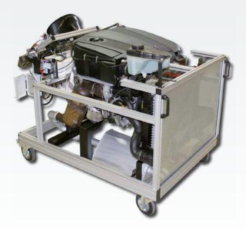
These fully operational engines ensure that none of the rotating parts are accessible and components which get hot are also covered over. Thus the working engines are very safe as well as being equipped with fault simulation. Signals from sensors and actuators can be accessed easily by means of break-out boxes.
