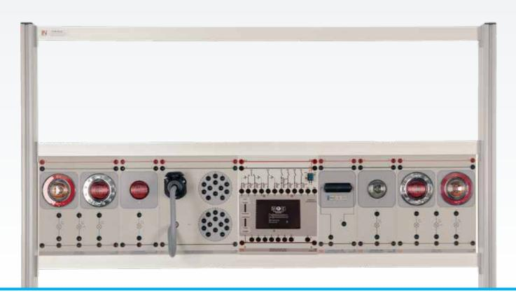
Teaching the topic of lighting for trailers has also become far more demanding in terms of the complexity of the electrical systems. The content imparted by the training system therefore goes beyond the principle of 7- or 13-pin plug connectors. It also explains how the towing vehicle is protected against overloading and when the control functions for the trailer meet regulations.
