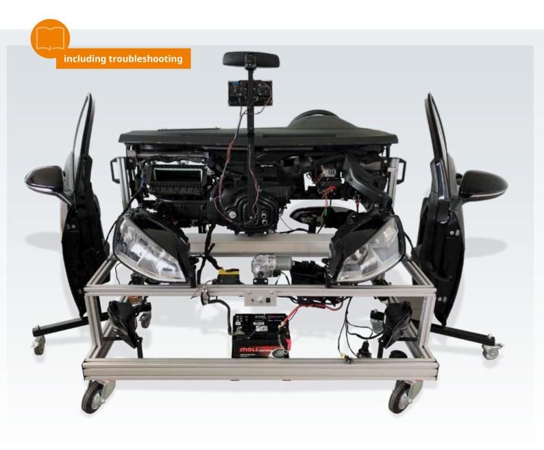
Carry out practical experiments using original components from a Volkswagen Golf 7, which is based on VW's MQB modular cross-component kits. This model for networked systems deals not only with the topics of actual CAN gateways but also covers the full electronic system for a steering column and includes fully functioning front doors with comfort controls.
