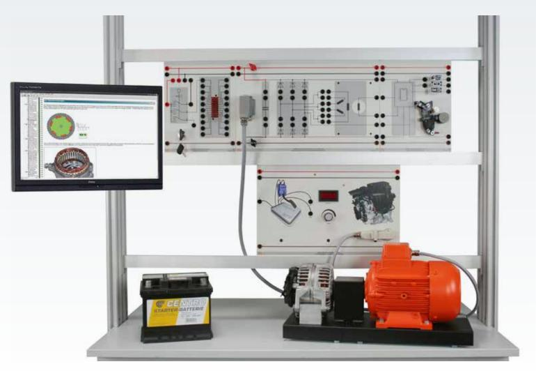
Today's compact generators make use of a monolithic controller. This kind of multifunction controller (MFC) has now largely replaced hybrid controllers. The training system shows how electrical energy is generated in modern vehicles with the help of experiments which build on one another.
