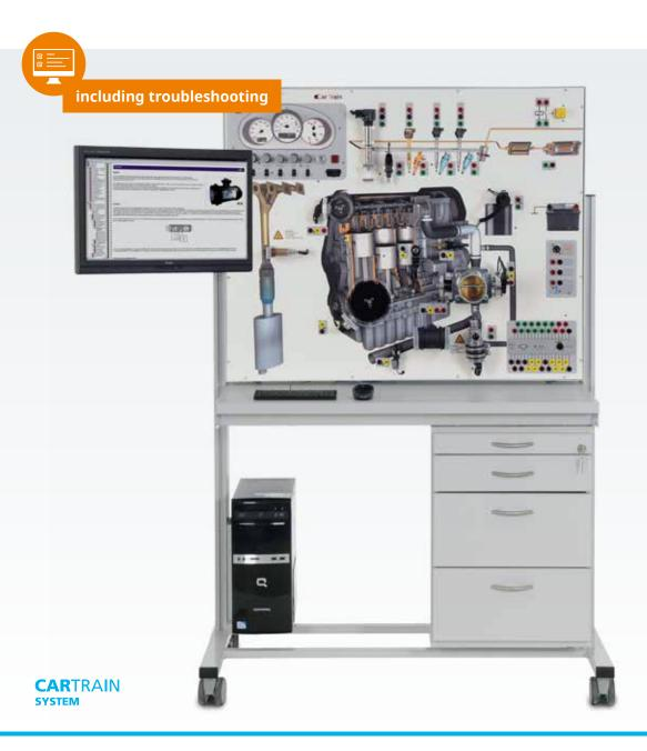
Our training system covering the Motronic 2.8.2 engine management system integrates all the management function (including preparation of fuel mix and ignition) into a single control unit. Each of the cylinders in a multi-point injection system has its own injection valve.
