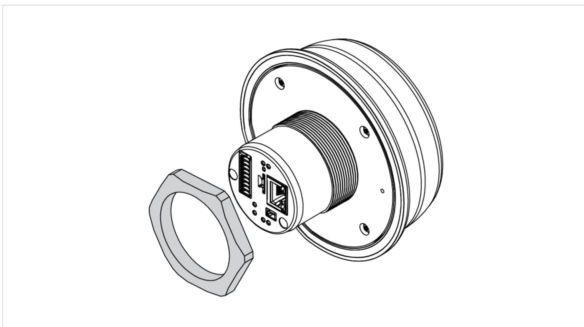
2. Place the Bolt 5G housing sealing ring in its groove.
