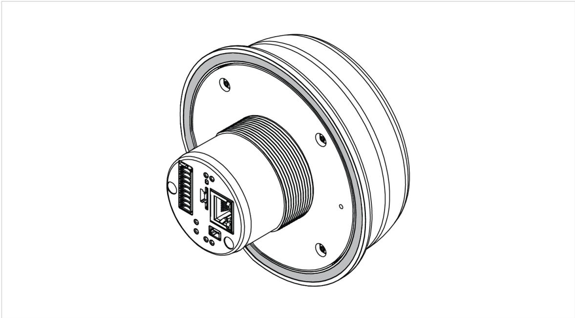
3. In the mounting surface, drill a mounting hole with the size  $\varnothing$  M50 (50,5 mm).
