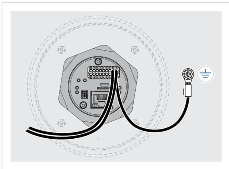
Figure 6. Functional earth wire screw placement, view from below
