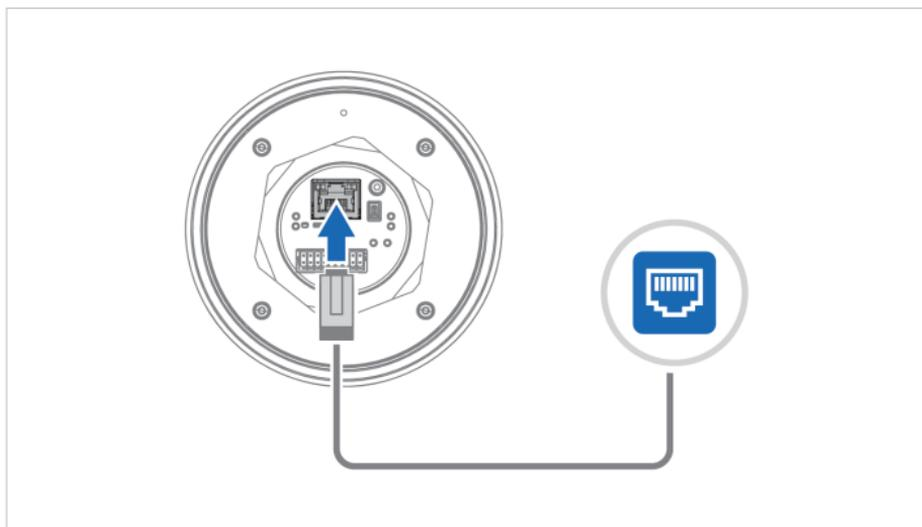
Figure 10. Connect to Ethernet
