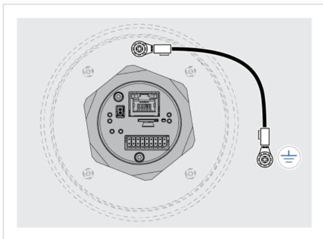
Figure 8. Functional earth wire screw placement, view from below
