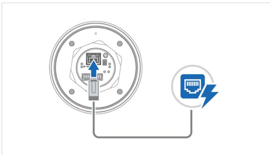
Figure 9. Connect to Power Over Ethernet (PoE)
