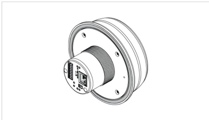
3. In the mounting surface, drill a mounting hole with the size  $\varnothing$  M50 (50,5 mm).
