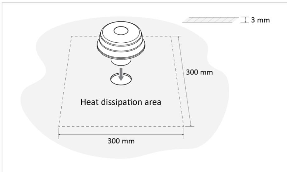
Figure 1. Mounting surface heat dissipation area
