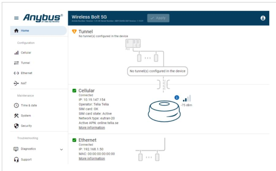
Figure 15. The Bolt 5G built-in web interface Home page
