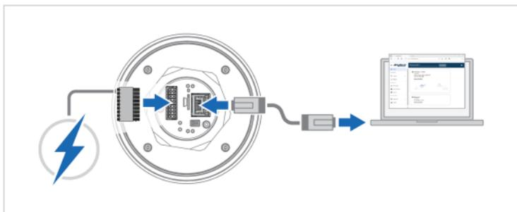
Figure 11. Connect to PC and Power
