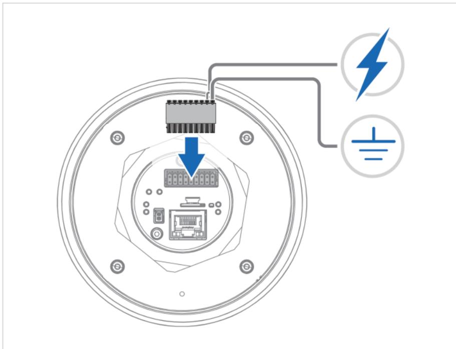
Figure 7. DC Power and Functional Earth (FE)
