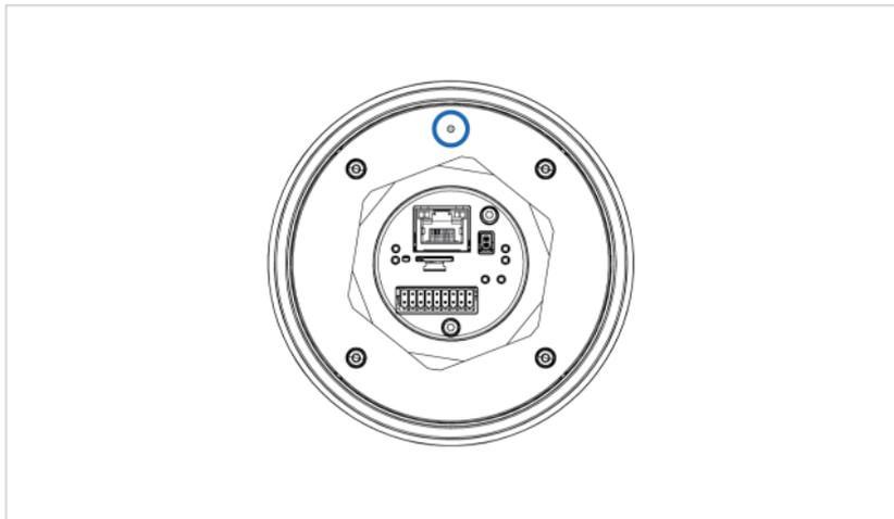
Figure 4. Bolt 5G steering hole for locking screw
