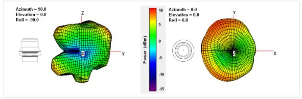
Fig. 27 2.4 GHz antenna gain and directivity in horizontal and vertical planes
