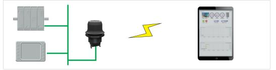
Fig. 25 Accessing a PLC from a handheld device using WLAN
