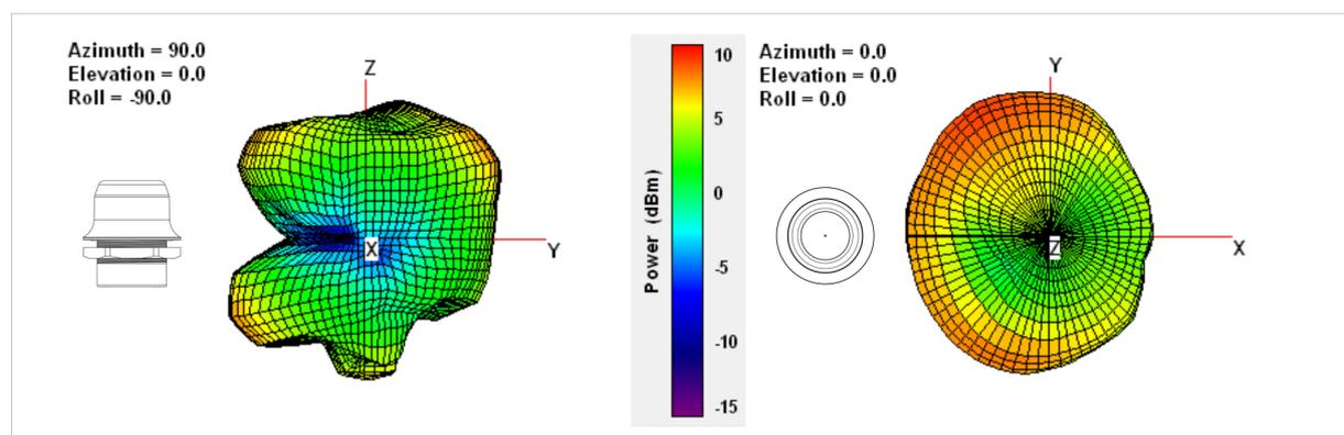
Fig. 27 2.4 GHz antenna gain and directivity in horizontal and vertical planes
