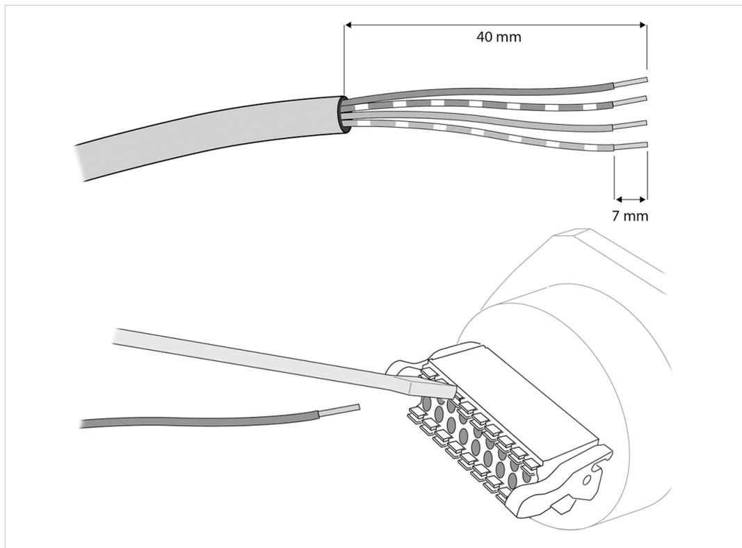
**Fig. 3 Ethernet cable**
