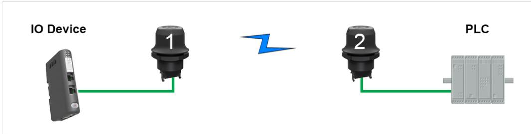
Fig. 22 EtherNet/IP wireless network
