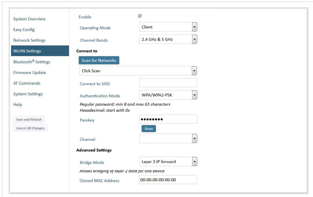
Fig. 8 WLAN Settings – Client
