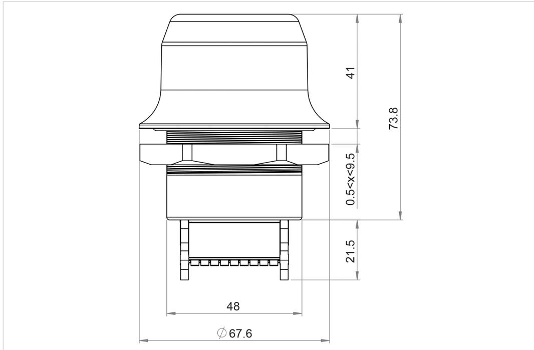
**Fig. 1** Installation drawing
