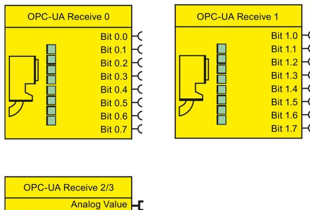
Figure 4-71 Schematic of the "OPC-UA Receive" function blocks
