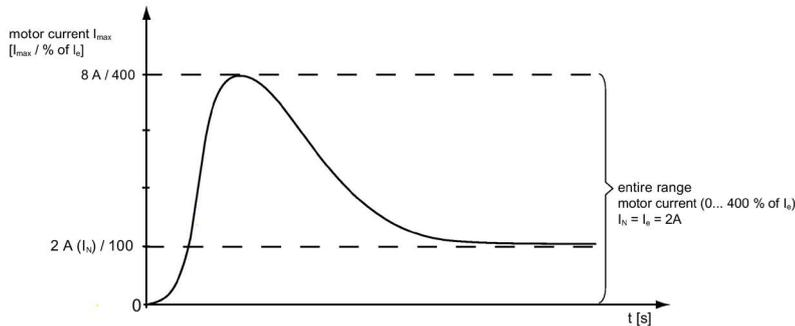
Figure 4-51 Application example: Motor current output - entire range
