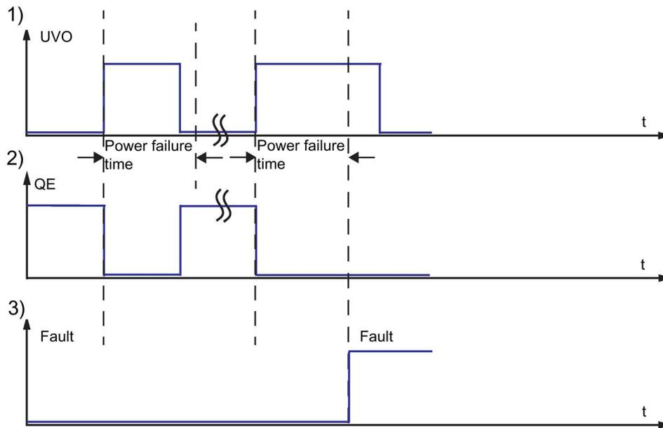
Figure 4-81 Power failure monitoring (UVO) sequence charts
