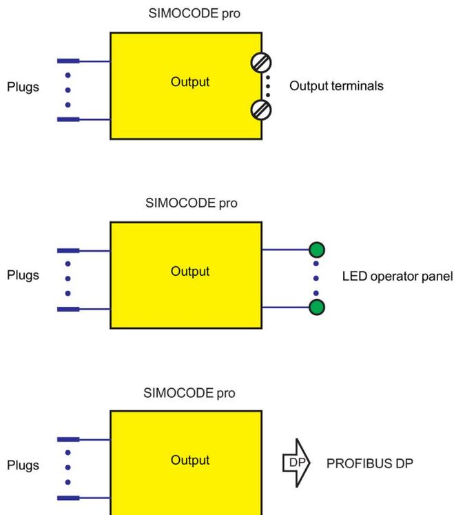
Figure 4-43 General representation of the various output types
