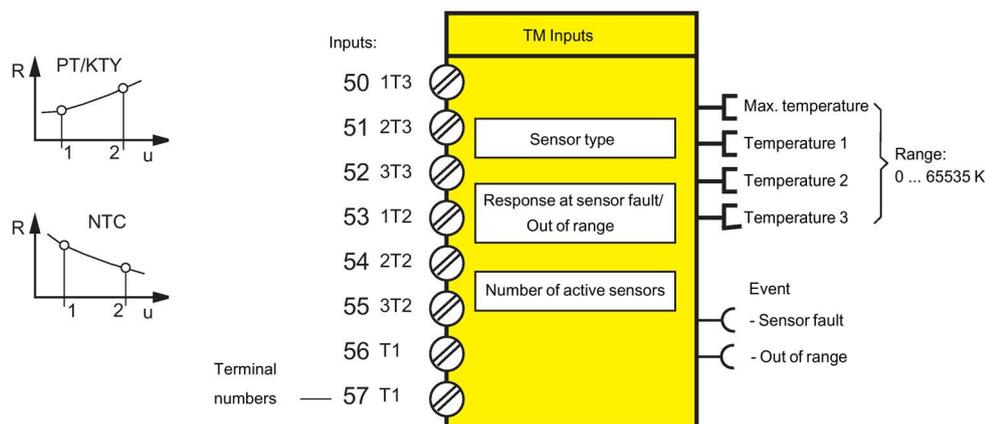
Figure 4-67 Schematic of the "TM Inputs" function block
