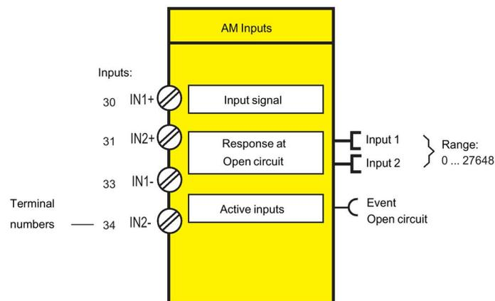
Figure 4-68 Schematic of the "AM1 Inputs" function block
