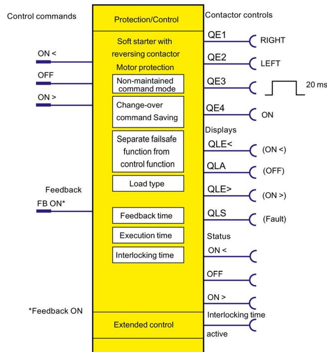
Figure 4-28 Schematic of the "Soft starter with reversing contactor" control function, "Protection / Control" function block
