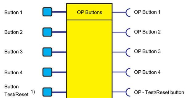
Figure 4-63 Schematic of the "OP Buttons" function block
