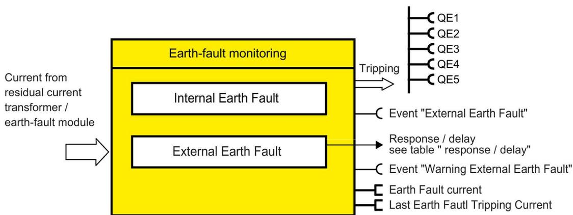
Figure 4-32 "Ground-fault Monitoring" function block
