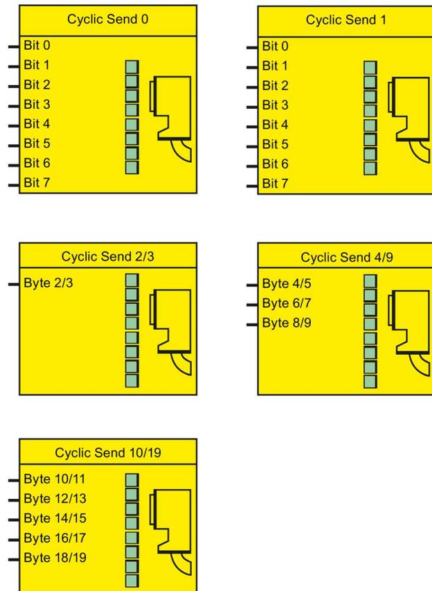
Figure 4-56 Schematic of the "Cyclic send" function blocks
