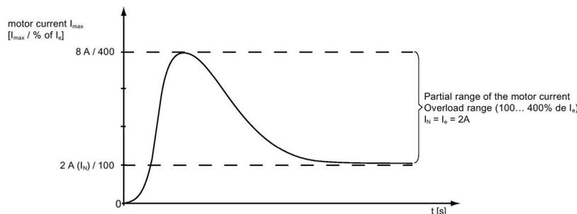
Figure 4-53 Application example: Motor current output - Overload range
