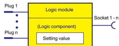
Figure 4-88 General representation of a logic module
