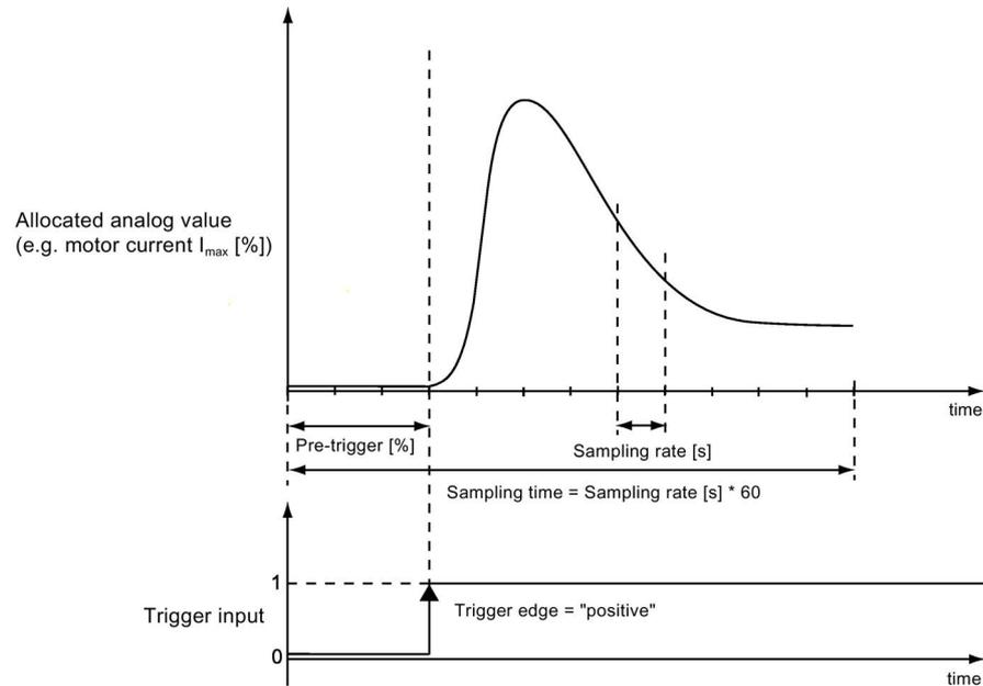
Figure 4-72 Analog value recording of measured curve
