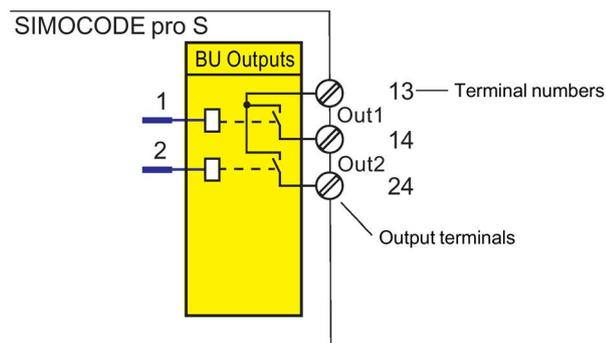
Figure 4-45 Function block "BU outputs," SIMOCODE pro S
