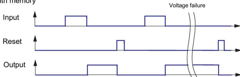
Figure 4-101 Types of signals / output responses of non-volatile elements
