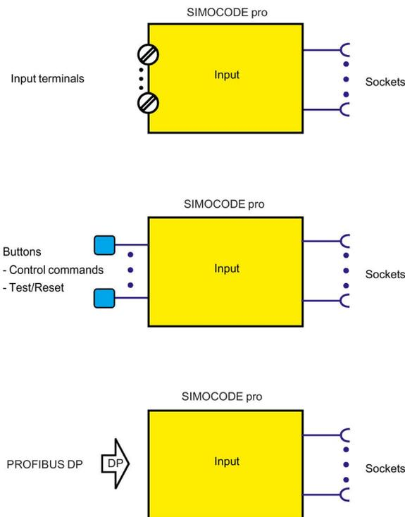
Figure 4-59 General representation of the input types
