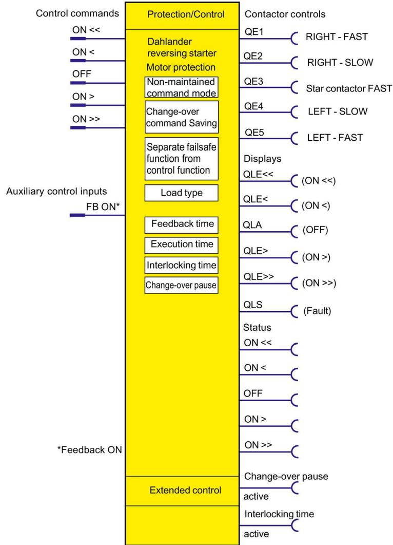
Figure 4-21 Schematic of the "Dahlander starter" control function, "Protection/Control" function block
