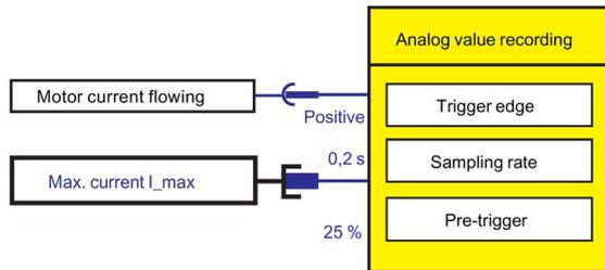
Figure 4-74 Application example of the analog value recording
