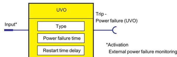
Figure 4-80 "Power Failure Monitoring (UVO)" function block
