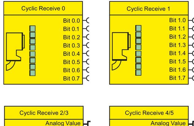
Figure 4-69 Function schematic of cyclic receive data
