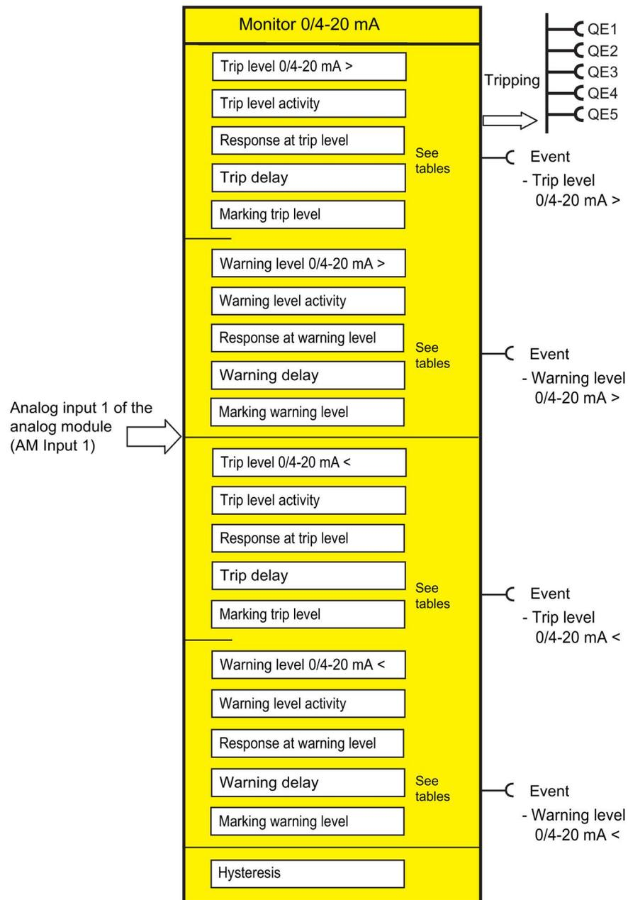
Figure 4-37 "0/4 to 20 mA monitoring" function block
