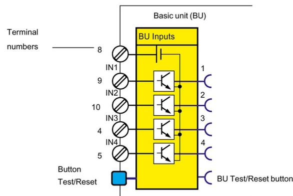
Figure 4-60 Schematic of the "BU Inputs" function block
