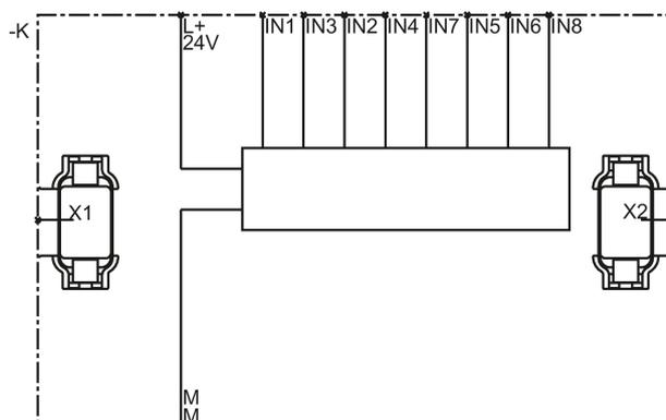
Figure 5-16 8-DI internal circuit diagram
