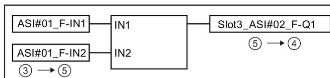
Figure 6-28 Setting/resetting of safety-related AS-i output in the logic diagram
