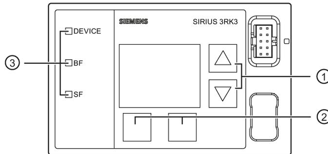
Figure 7-10 Display and operating elements on the diagnostics display
