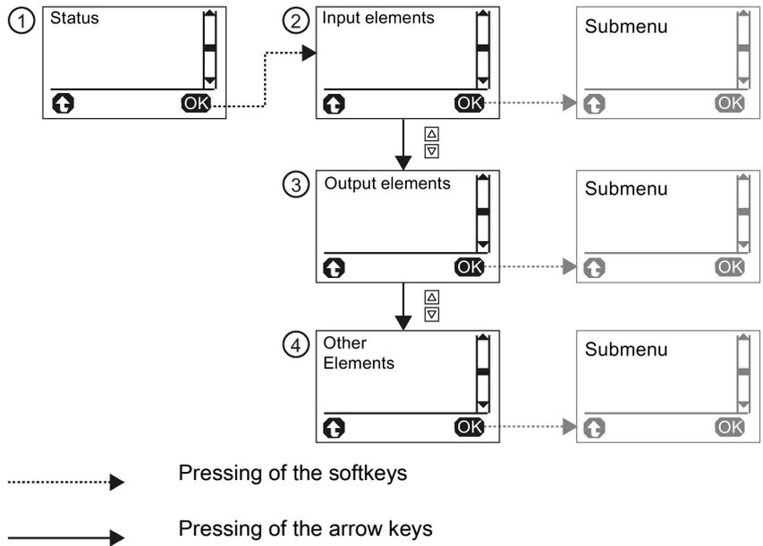
Figure 7-13 Second level of the menu of the diagnostics display - "Status" menu option
