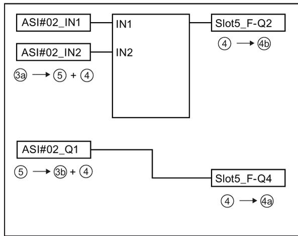
Figure 6-37 Evaluation of the safety-related AS-i input slaves and of the standard outputs in the logic diagram
