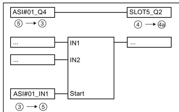
Figure 6-33 Evaluation of the non-safety-related AS-i slave in the logic diagram
