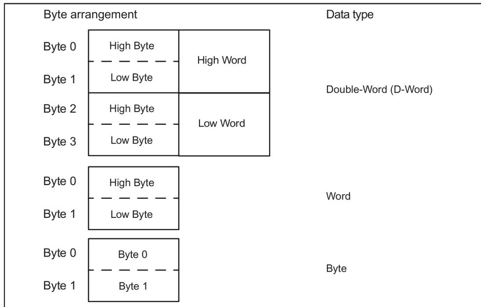
Figure 7-2 Byte arrangement
