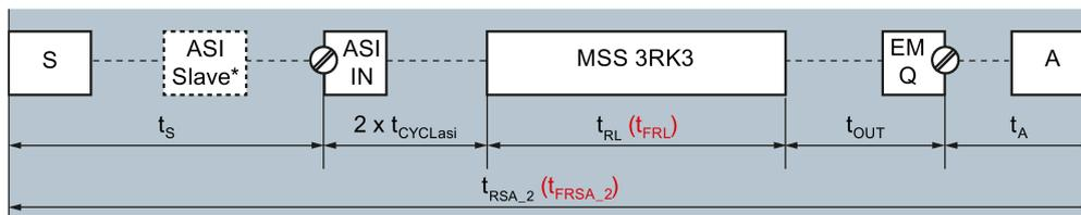
Figure 6-11 Reaction times MSS 3RK3 Advanced - example 2
