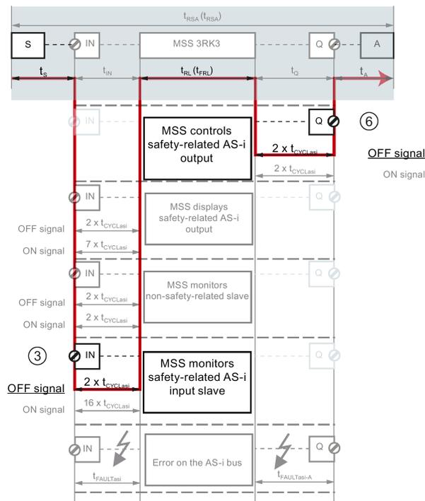
Figure 6-7 Signal flow of example 1
