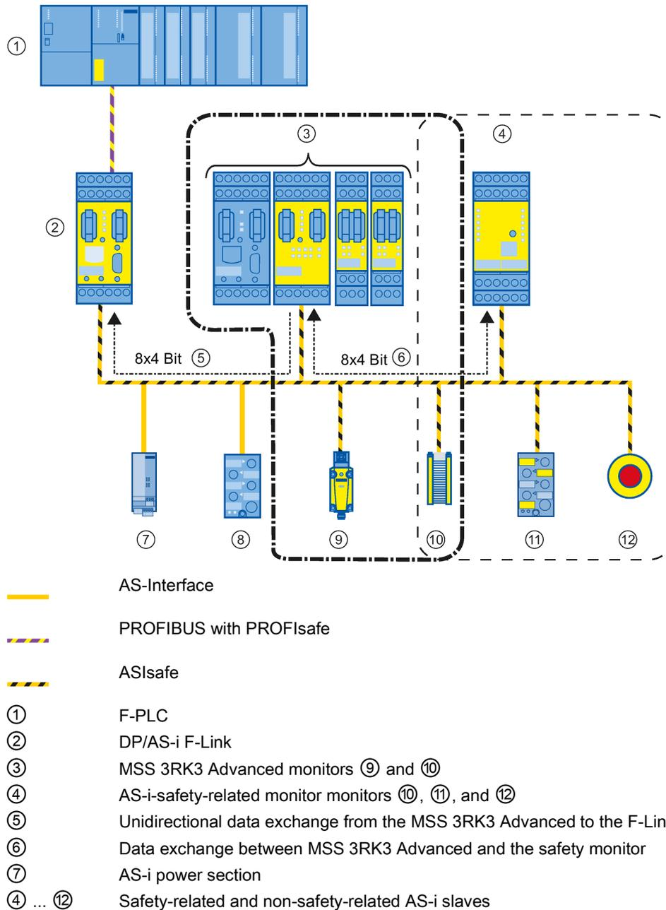
Figure 6-22 AS-Interface with different subnetworks
