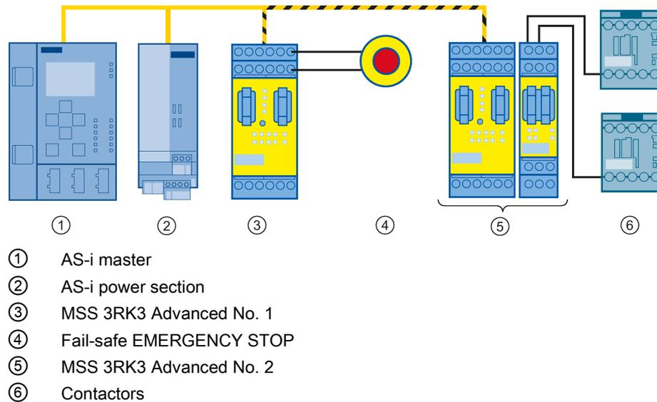
Figure 6-12 Configuration MSS 3RK3 Advanced - example 3
