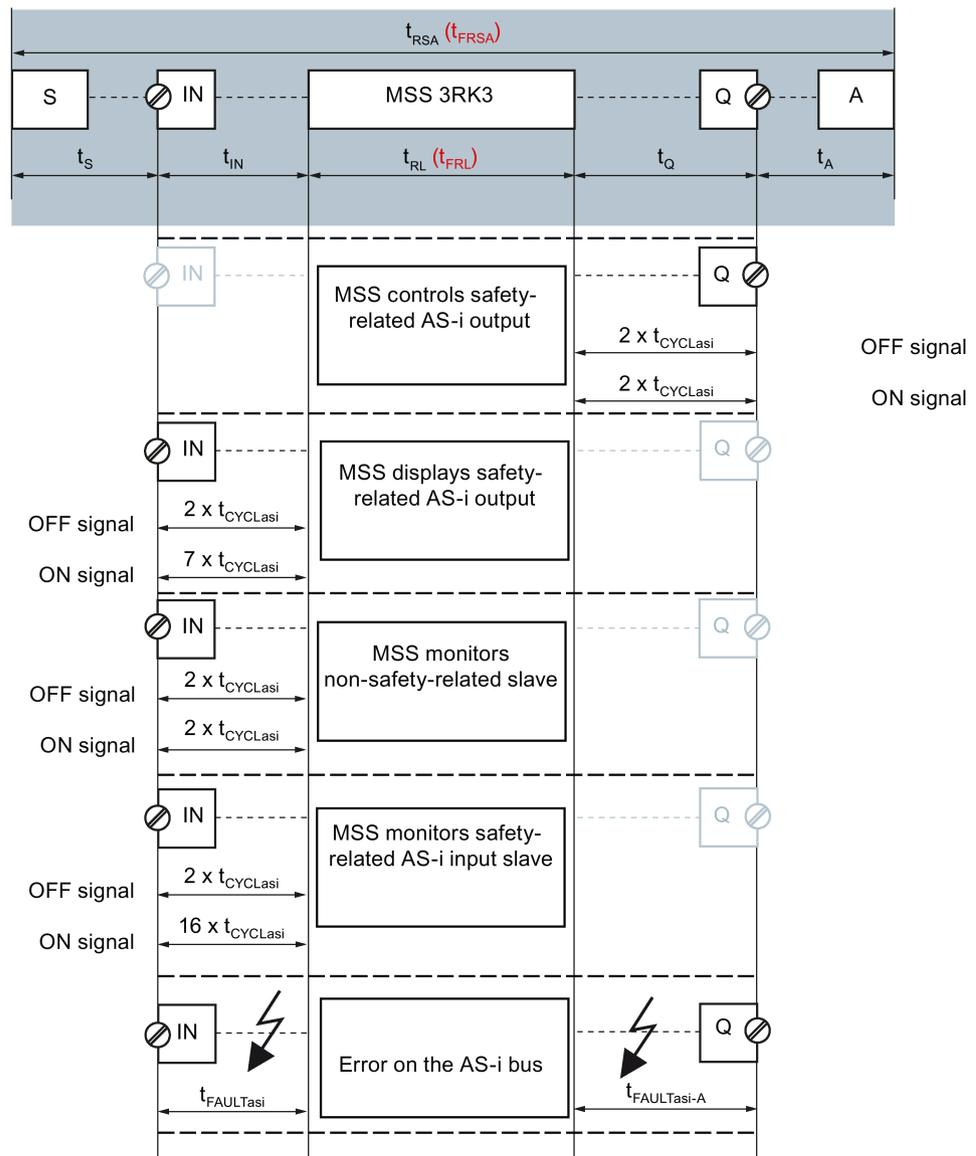
Figure 6-5 Reaction times "sensor - actuator" - Part 2
