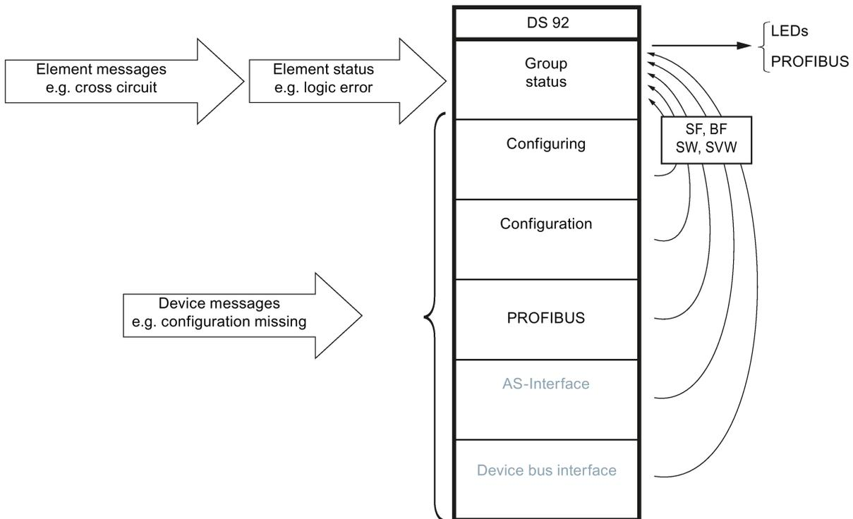
Figure 7-1 MSS 3RK3 diagnostics concept
