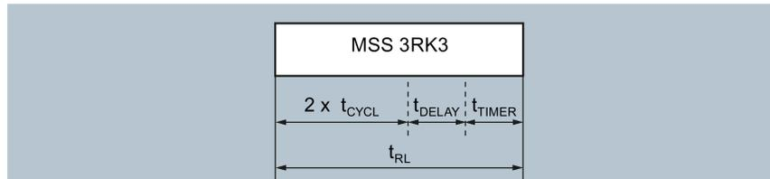
Figure 6-1 Reaction time of the logic (in error-free operation)
