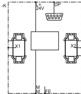
Figure 5-19 DP interface internal circuit diagram
