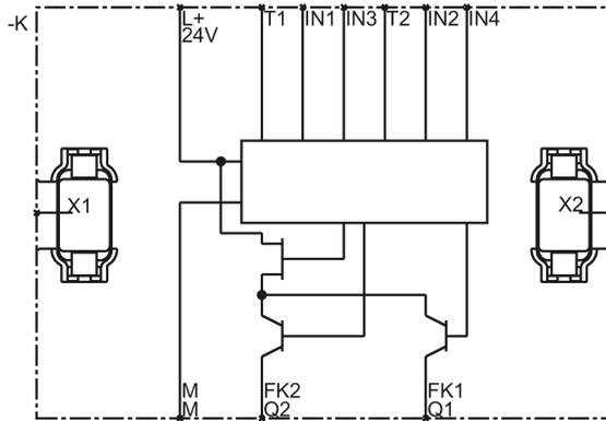
Figure 5-13 2/4F-DI 2F-DO internal circuit diagram
