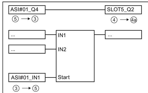
Figure 6-35 Evaluation of the safety-related AS-i input slave in the logic diagram
