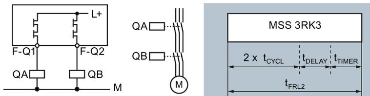
Figure 6-3 Fault reaction time of the logic for a two-channel actuator circuit
