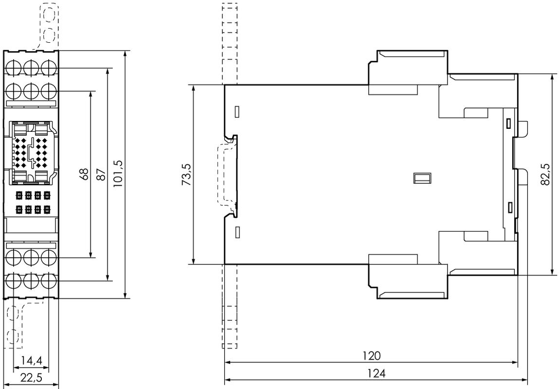
Dimension drawing of 22.5-mm enclosure with spring-loaded terminals
