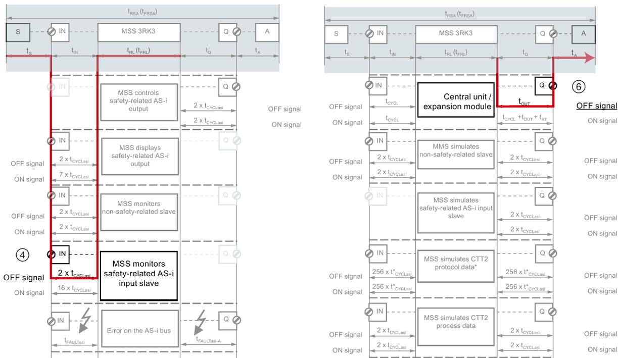
Figure 6-10 Signal flow of example 2
