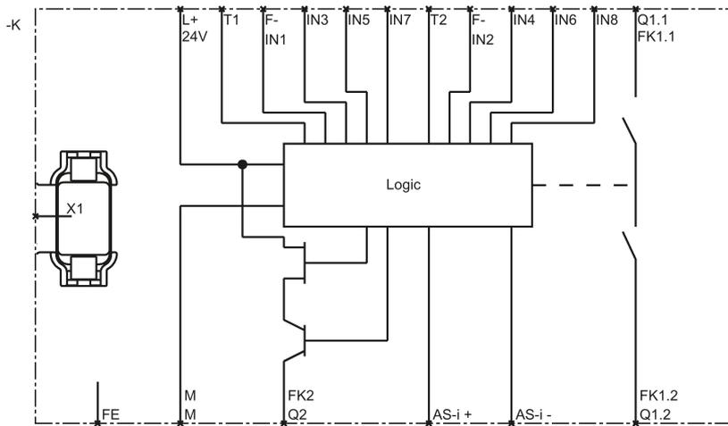
Figure 5-7 MSS 3RK3 ASIsafe basic internal circuit diagram
