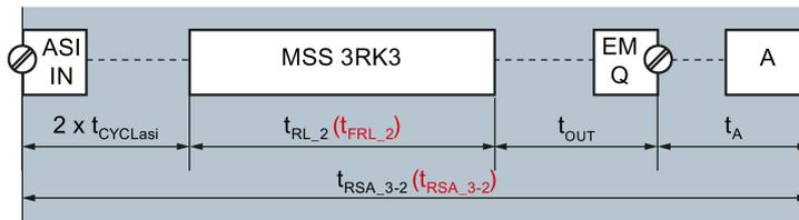
Figure 6-16 Reaction times MSS 3RK3 Advanced No. 2 - example 3
