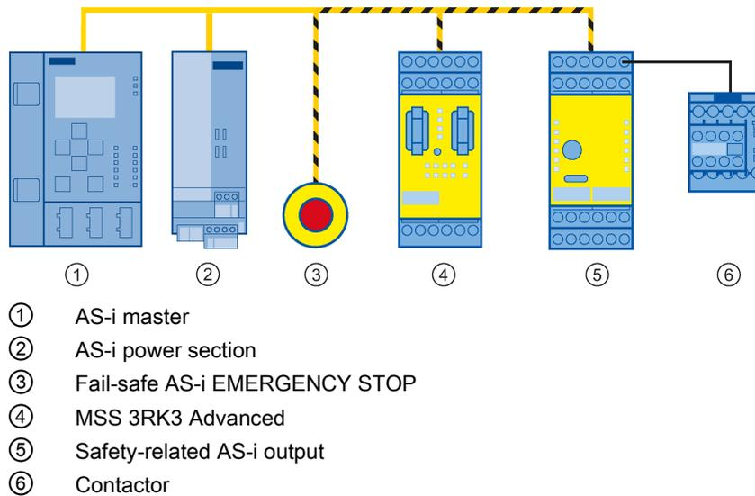
Figure 6-6 Configuration MSS 3RK3 Advanced - example 1
