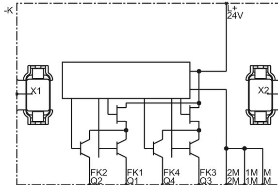
Figure 5-14 4F-DO internal circuit diagram
