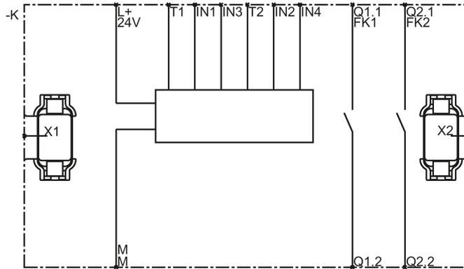
Figure 5-12 2/4F-DI 1/2F-RO internal circuit diagram
