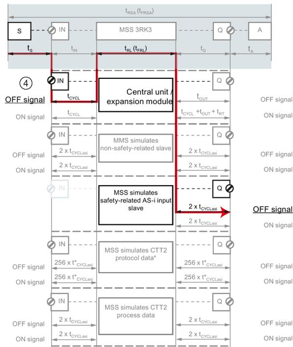
Figure 6-13 Signal flow of example 3 for MSS 3RK3 Advanced No. 1
