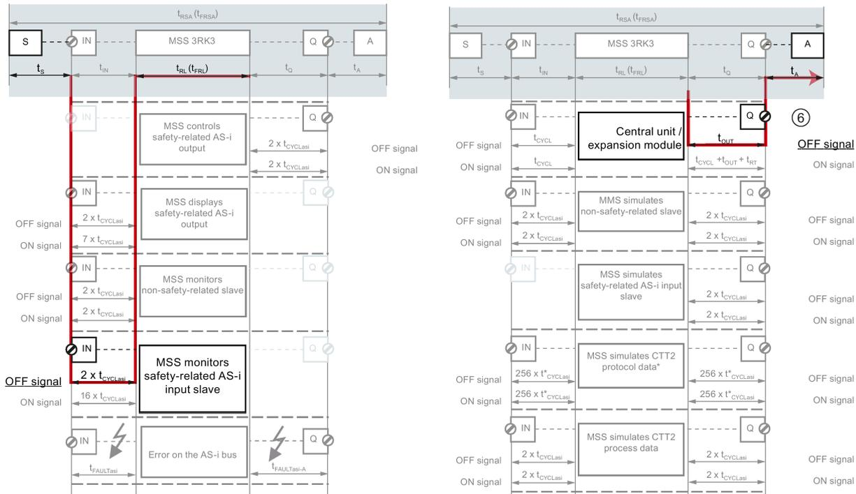
Figure 6-15 Signal flow of example 3 for MSS 3RK3 Advanced No. 2
