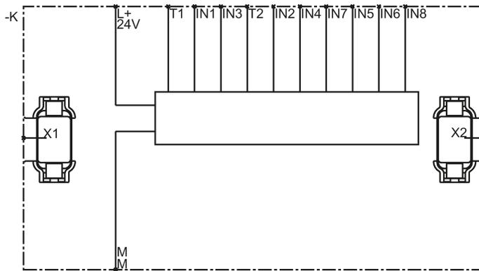
Figure 5-11 EM 4/8F-DI internal circuit diagram
