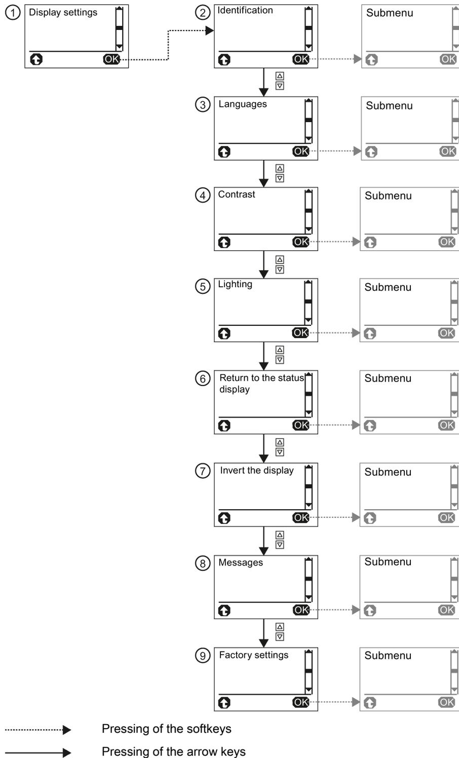
Figure 7-15 Second level of the menu of the diagnostics display - "Display settings" menu option
