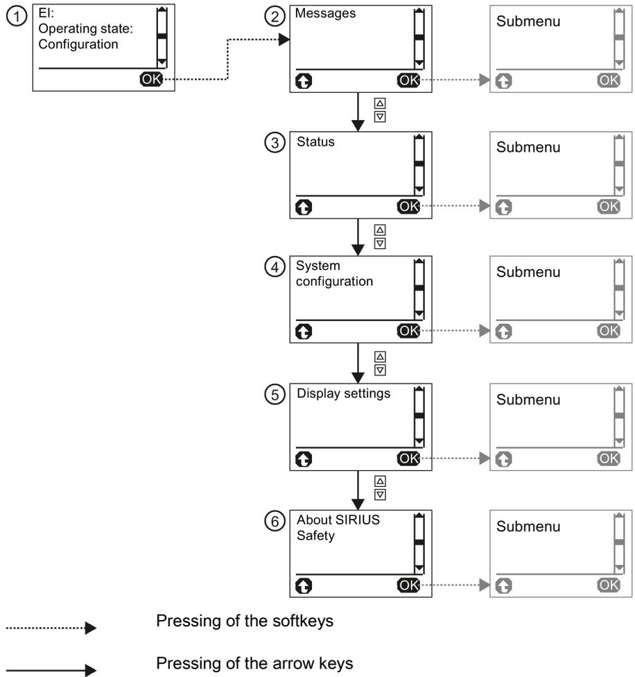
Figure 7-11 First level of the menu of the diagnostics display
