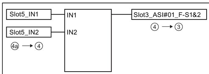
Figure 6-26 Simulation of safety-related AS-i input slaves in the logic diagram
