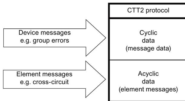
Figure 7-4 Diagnostics concept of MSS 3RK3 with AS-i interface using CTT2
