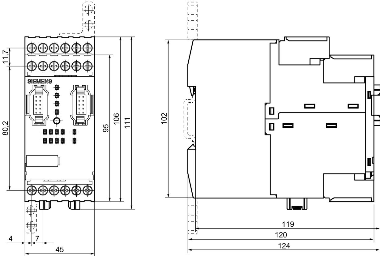
Dimension drawing of 45-mm enclosure with spring-loaded terminals
