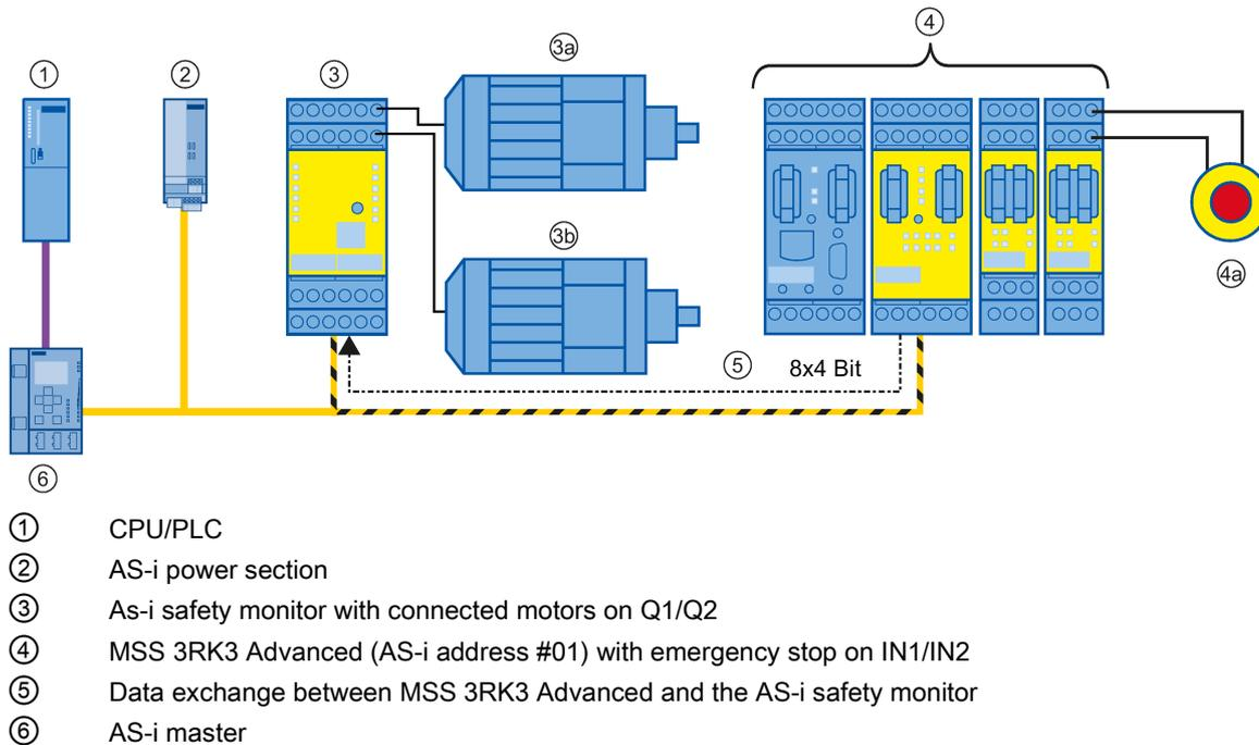
Figure 6-25 Simulation of safety-related AS-i input slaves
