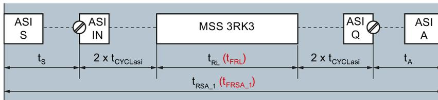
Figure 6-8 Reaction times MSS 3RK3 Advanced - example 1
