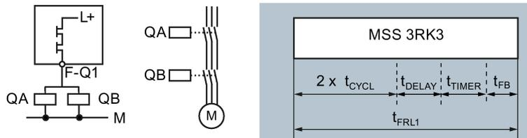
Figure 6-2 Fault reaction time of the logic for a single-channel actuator circuit
