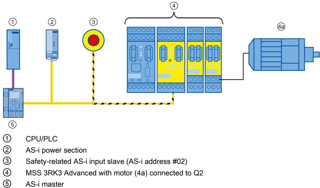
Figure 6-34 Evaluation of a safety-related AS-i input slave
