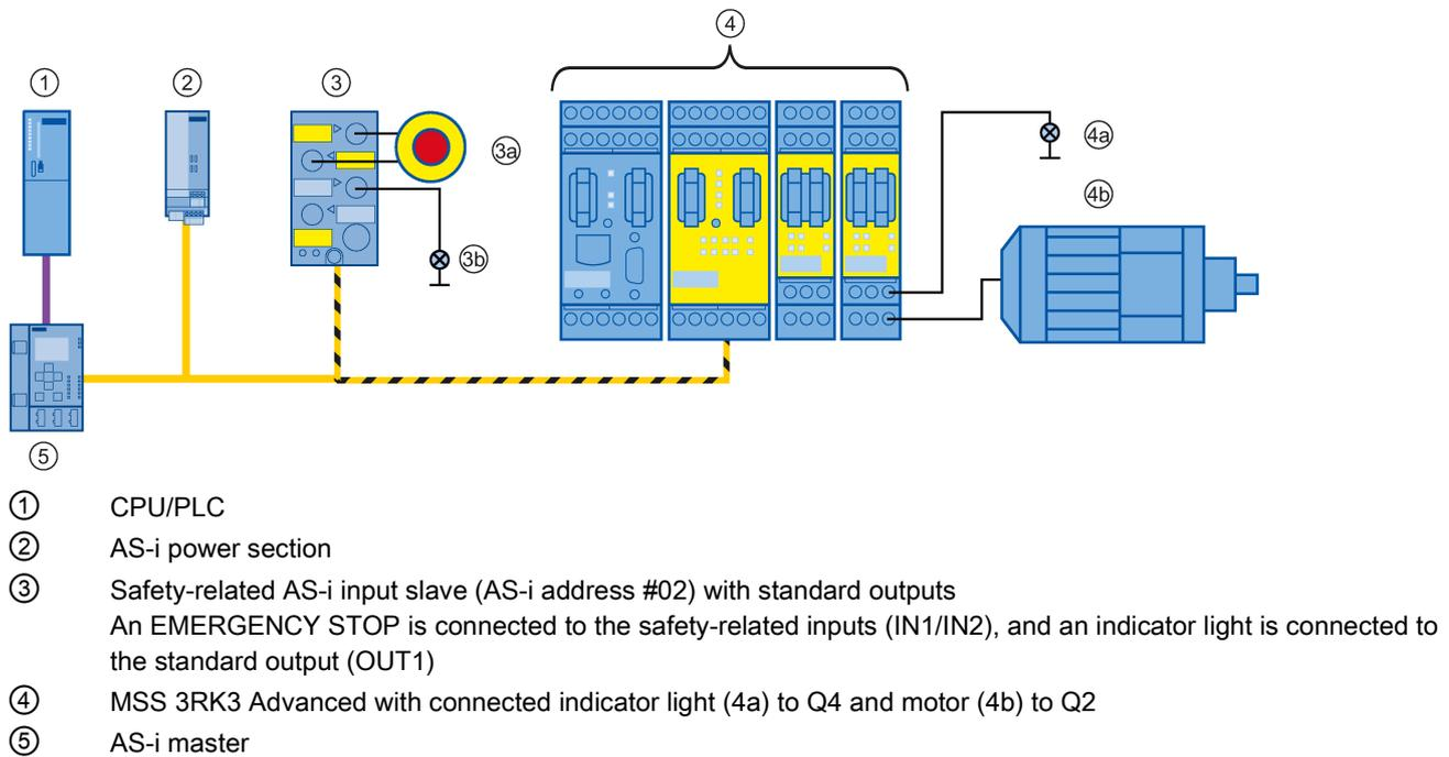
Figure 6-36 Evaluation of a safety-related AS-i input slave
