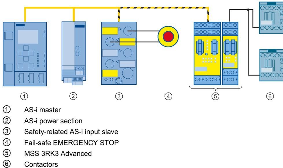
Figure 6-9 Configuration MSS 3RK3 Advanced - example 2
