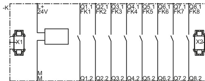
Figure 5-15 4/8F-RO internal circuit diagram
