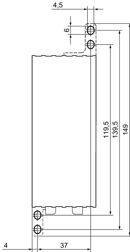
Dimension drawing: Enclosure 22.5 mm with screw terminals
