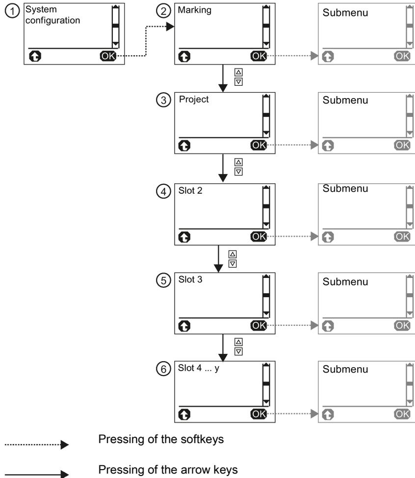
Figure 7-14 Second level of the menu of the diagnostics display - "System configuration" menu option
