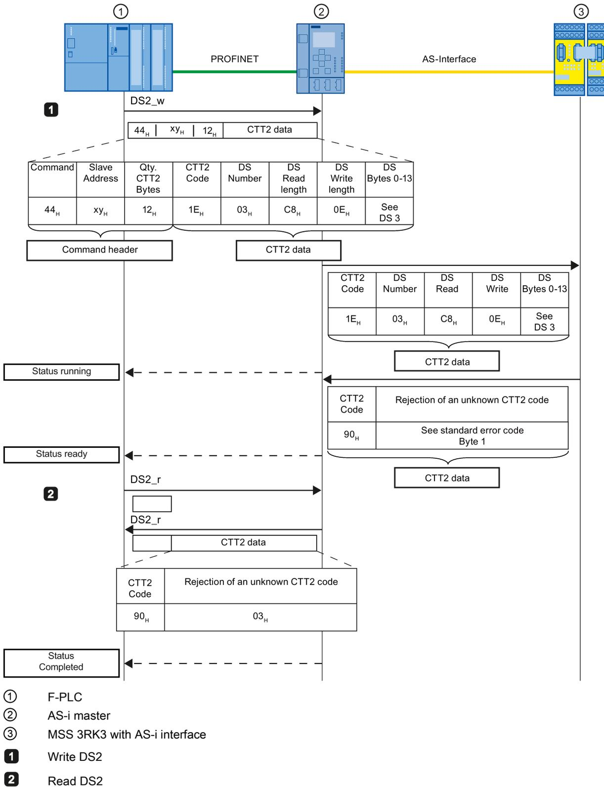
Figure 7-7 Example of transmission with error because of incorrect CTT2 code
