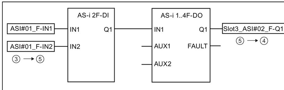
Figure 6-29 Controlling safety-related AS-i outputs using function element AS-i 1..4F-DO
