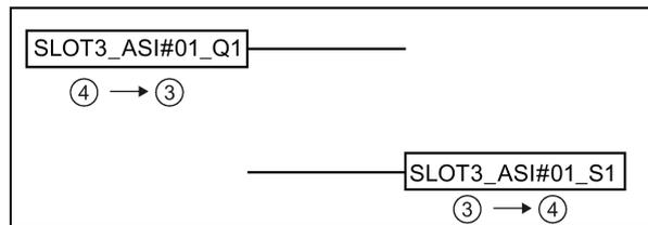
Figure 6-24 Simulation of non-safety-related AS-i slaves in the logic diagram
