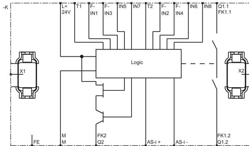
Figure 5-9 MSS 3RK3ASIsafe extended internal circuit diagram
