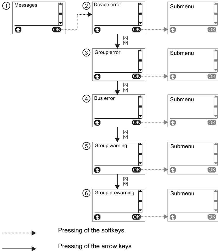
Figure 7-12 Second level of the menu of the diagnostics display - "Messages" menu option
