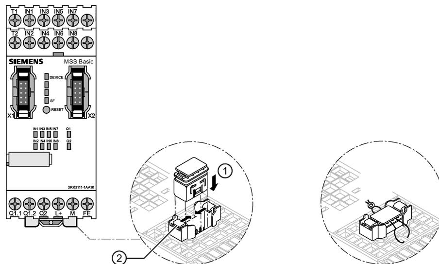
Figure 5-24 Connecting the memory module
