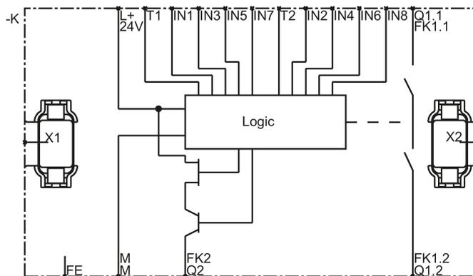
Figure 5-3 MSS 3RK3 Basic internal circuit diagram
