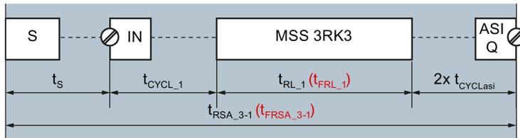
Figure 6-14 Reaction times MSS 3RK3 Advanced No. 1 - example 3
