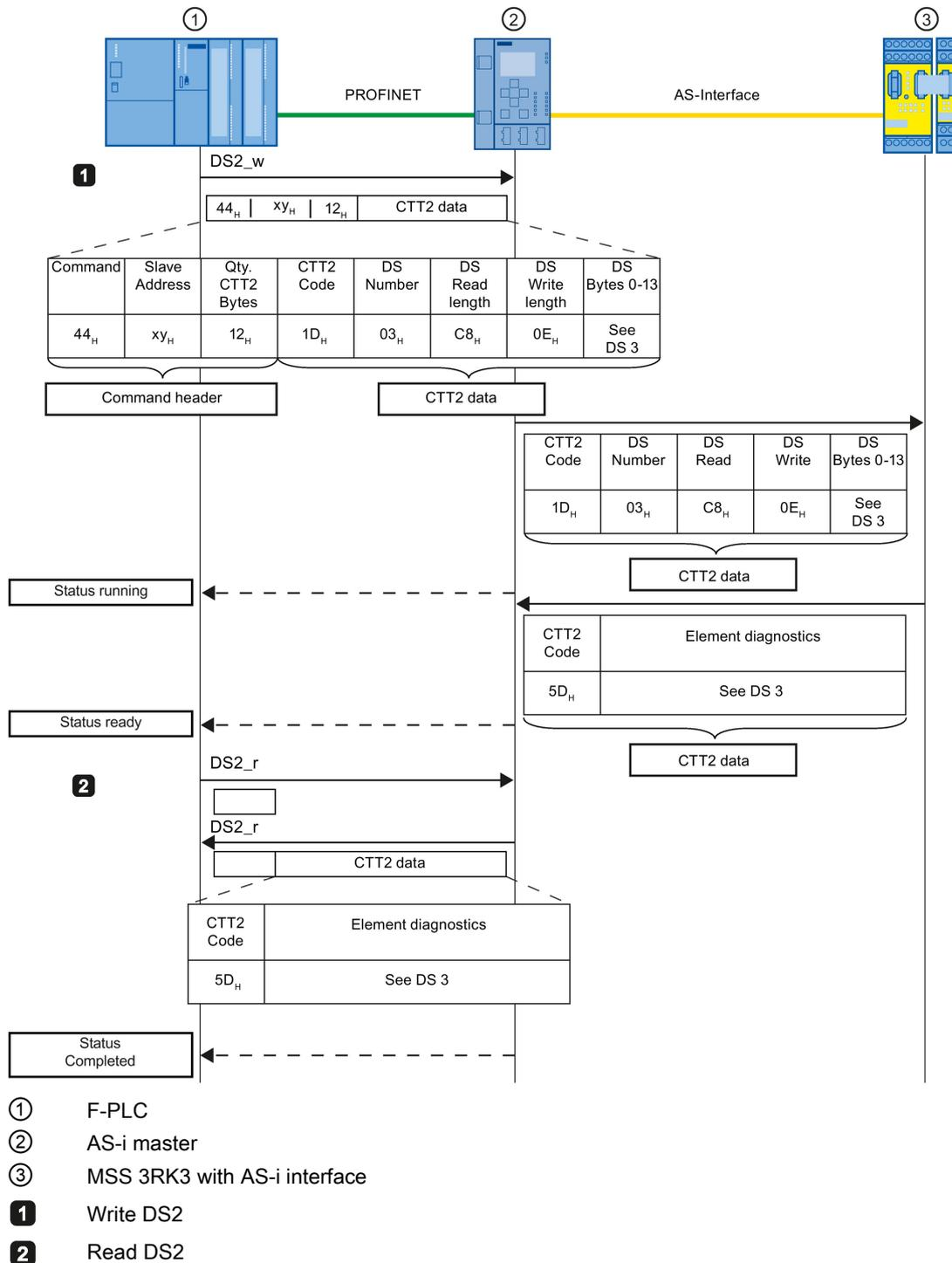
Figure 7-5 Example of transmission without error
