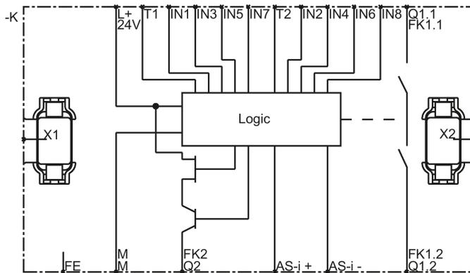
Figure 5-5 MSS 3RK3 Advanced internal circuit diagram
