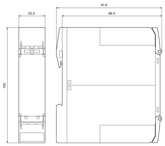
Figure 14-3 Enclosure 22.5 mm (short) for safety relays: 3SK1112-.....
