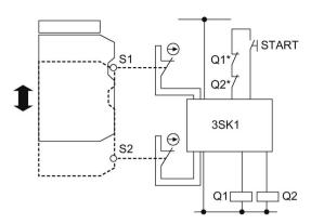
Figure 4-2 Two-channel sensor connection
