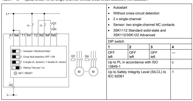
Also possible: 2 x single-channel with T1-IN1, T2-IN2 and DIP switch 2 cross-circuit detection to ON.
