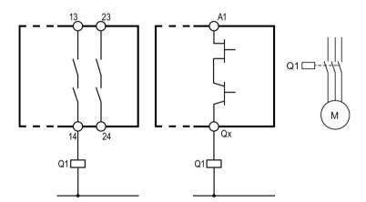
Figure 4-5 PL c / Cat. 2 in accordance with ISO 13849-1 or SILCL 1 in accordance with IEC 62061
