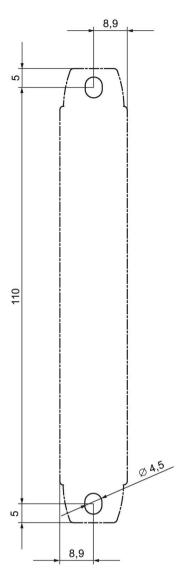
Figure 14-2 Drilling diagram, enclosure 17.5 mm
