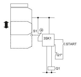
Figure 4-1 Single-channel sensor connection
