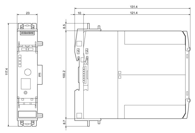
Figure 14-6 3SK1 device on device connector
