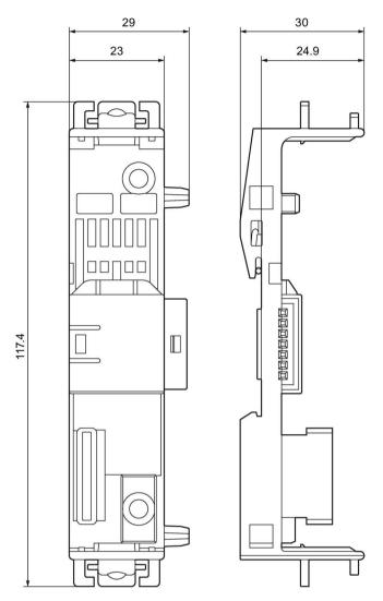
Figure 14-13 Device connector for 3RM1 motor starters, width: 22.5 mm
