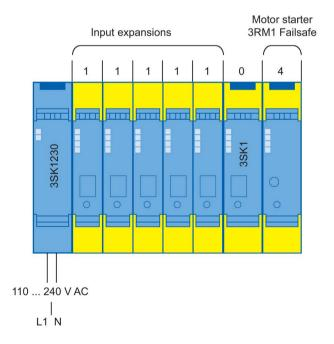
Example 3) 1 x 3SK1230 power supply; 2 x 3SK1220 input expansion; 1 x 3SK112 basic unit; 2 x 3RM1 Failsafe motor starter
