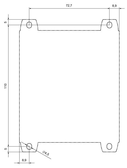
Figure 14-8 Drilling diagram, enclosure 90 mm
