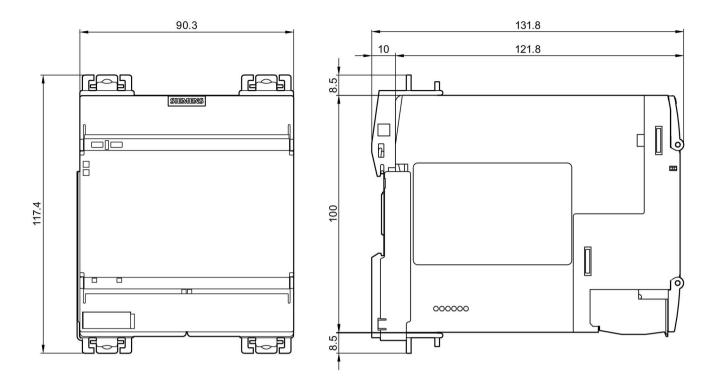
Figure 14-9 3SK1213 device on device connector
