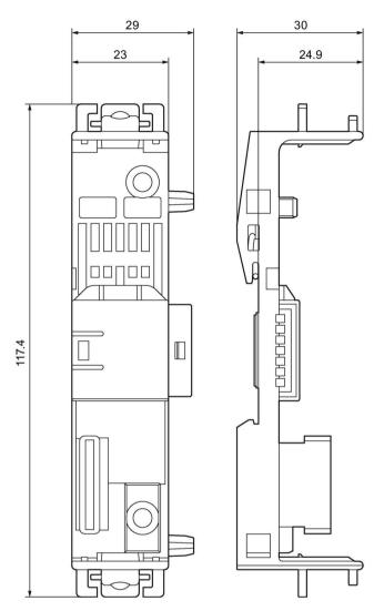
Figure 14-11 Device connector for 3SK1 safety relays, width: 22.5 mm
