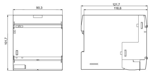
Figure 14-7 Enclosure 90 mm for safety relays: 3SK1213-.....
