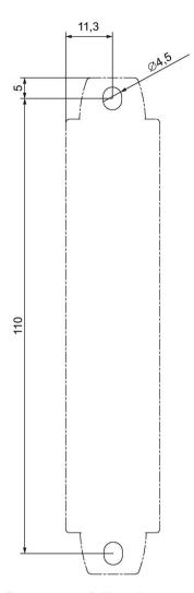
Figure 14-5 Drilling diagram, enclosure 22.5 mm
