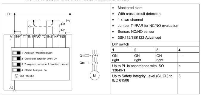
Table 7- 15 Typical circuit 15: 1NC/1NO sensor, with cross-circuit detection, with autostart
