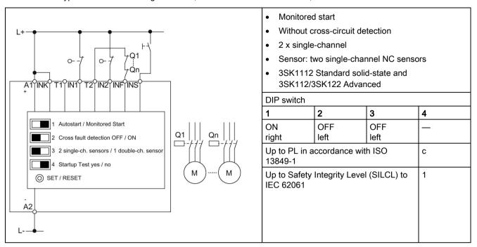
Table 7- 13 Typical circuit 13: 2x single-channel, without cross-circuit detection, with autostart
