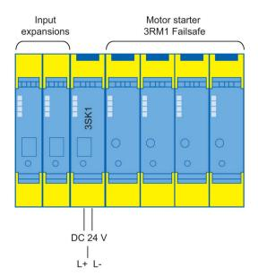
Example of a configuration with connection of 24 V DC on the basic unit and 3RM1 Failsafe motor starter
