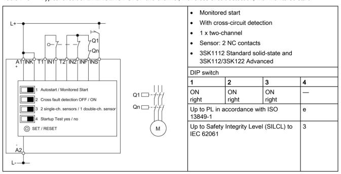
Table 7-9 Typical circuit 9: Two-channel, with cross-circuit detection, with autostart
