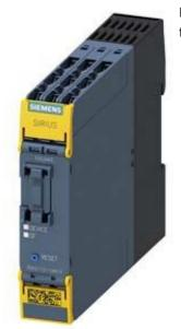
SIRIUS safety relay Basic unit 3SK2 series 10 F-DI, 2 F-DQ, 1 DQ, 24 V DC Can be parameterized via SIRIUS Safety ES 22.5 mm overall width screw terminal up to SILCL 3 (DIN EN 62061) Up to Performance Level E (ISO 13849-1) Output expansions 3SK1 and fail-safe motor starters 3RM1 via device connector connectable
